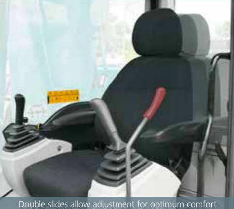
Double slides allow adjustment for optimum comfort
