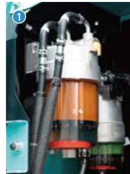
1 Pre-filter with integrated water separator
