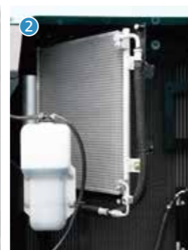
2 Openable air conditioner condenser Easy to clean inside
