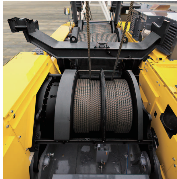
View towards the front of the machine : Front, Rear and Boom drums
