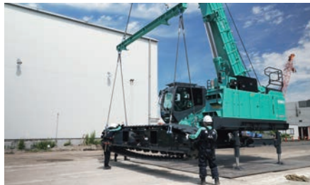
Crawlers can be self-mounted and removed using a special suspension balance, with a working radius of up to 5.5m.
