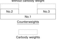
Although, the total weight of the counterweight is different between machine equipped with self-removal device (optional type) and machine not equipped with self-removal device (standard type), the lifting capacity is the same.
