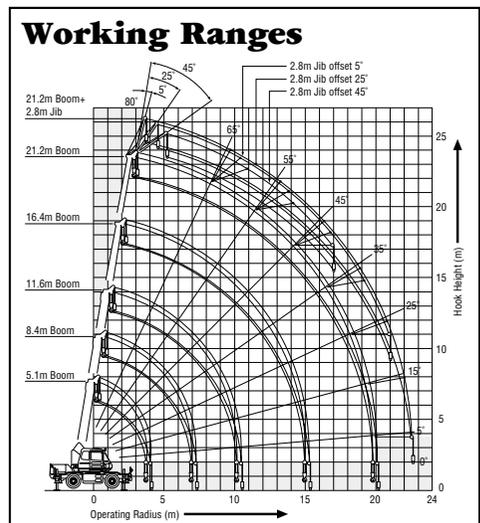
\*Boom/jib bending with load is not involved in figure of working ranges.
