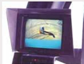
Cameras monitor the drums to help the operator catch potential accidents, such as spooling malfunctions, in their early stages. The cameras also monitor the rear of the machine to ensure the safety of workers
