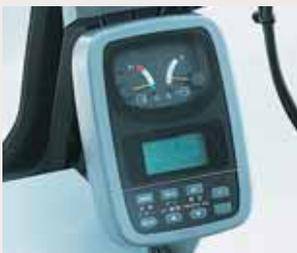
The LCD multi-display shows a malfunction log (including fuel, hydraulic oil, cooling water, etc.) for 16 items, and its self-diagnostic function monitors a total of 41 items, including electrical malfunctions involving solenoid valves, sensors, etc.
