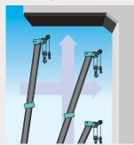
By setting the parameters of boom angle (upper and lower limits), boom top height, and operating radius, the operator can limit the range in which the boom operates. A warning buzzer sounds and the machine stops automatically whenever those limits are approached. This mechanism has proved successful on
