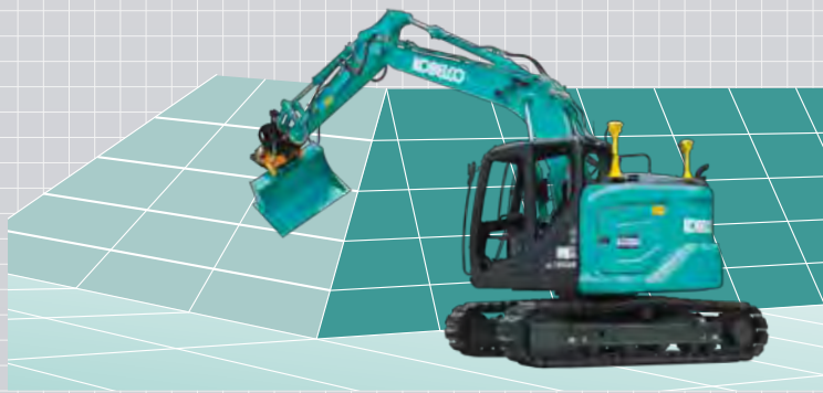
One of the Dig Nav products: 3D-tilt machine control system
