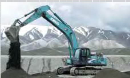
Engine high altitude test at an altitude of 4,310m
